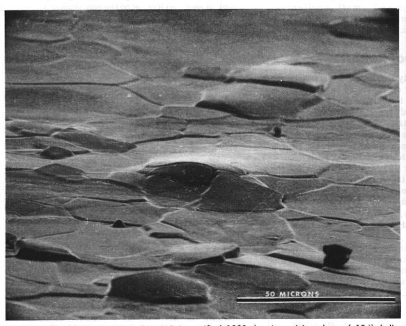
MICROGRAPH OF PALLADIUM SAMPLE (magnified 1000 times) receiving dose of 10 17 helium atoms per square centimeter at an energy level of 5 MeV shows grains that have been forced up from the surface and tilted at various angles. One dome includes several grains whose boundaries have split open. These features were not seen in samples receiving doses below 10 16 helium atoms/cm2. Unusual helium release phenomenon indicated outgassing was dependent on the helium concentration in the sample.
